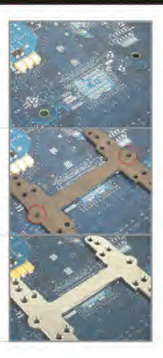
Insert the screws through the holes as shown.
